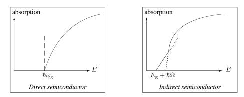
So indirect semiconductors, like Si and Ge, cannot emit any light and are therefore not usable to fabricate lasers. When light is absorbed holds:  $\vec{k}_{\rm h} = -\vec{k}_{\rm e}$ ,  $E_{\rm h}(\vec{k}_{\rm h}) = -E_{\rm e}(\vec{k}_{\rm e})$ ,  $\vec{v}_{\rm h} = \vec{v}_{\rm e}$  and  $m_{\rm h} = -m_{\rm e}^*$  if the conduction band and the valence band have the same structure.
